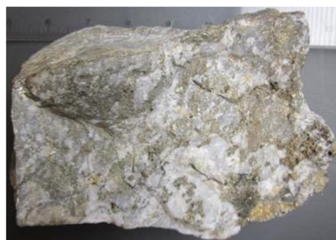
Typical Ore Sample (Qtz-Py-Au Vein)
