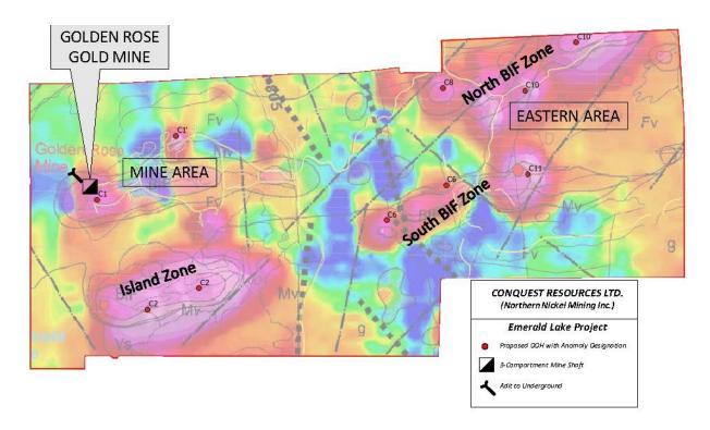
Figure 1: VTEM geophysical map showing exploration zones and recommended diamond drill holes
