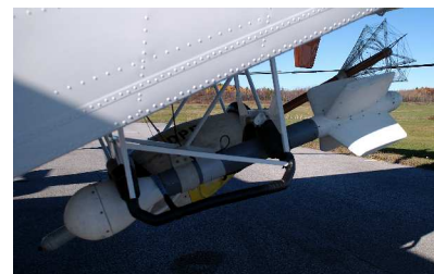
Figure 3: Mag and GEOTEM® Receivers
